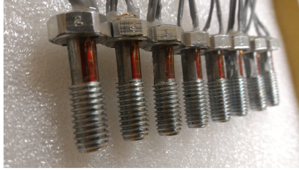
Figure 5: Bolts instrumented with strain gauge.
