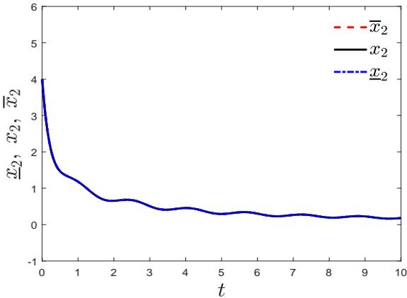
Fig. 2. The interval  $[x_2, \bar{x}_2]$  estimated by the observer (5) with (24) and (26) for plant (1) given by (23) with initial condition (29) and disturbance (30); The three lines completely overlap.
