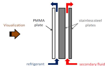
Figure 2: Scheme of the evaporator (from Giraud, 2016)
