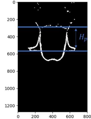
Figure 6b: calculation of the projection height (pixels)
