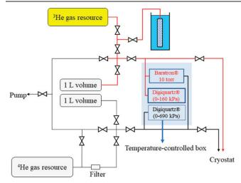
**Figure 3.** Gas handling system for  ${}^{3}$ He vapour–pressure measurements (red lines). The 1 L volumes are used to estimate the amount of helium in either or both of the evaporators, this volume being a few times greater than that of the rest of the tubing.
