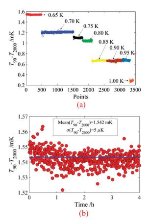
**Figure 11.** (a) The stability of  $T_{90}-T_{2000}$  at each temperature point b) Enlargement for 650 mK. Note that data for each temperature were obtained on different days.
