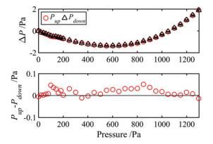
**Figure 8.** The calibration of the capacitance manometer  $CM_{VPT}$  (MKS Baratron 698A) used to measure <sup>3</sup>He pressure with respect to a piston balance (Fluke FPG8601) traceable to the French national standard.
