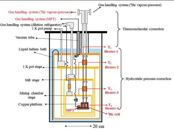
**Figure 1.** The cryostat used for the comparison of the temperature scales ITS-90 and PLTS-2000. MPT: melting-pressure thermometer. The gas handling system for <sup>4</sup>He is not used in the present work. For a detailed description see Sparasci *et al* (2011) [23]. For convenience, the vertical scale has been compressed.
