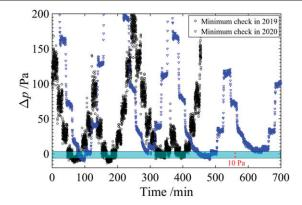
**Figure 6.** Minima of the melting pressure recorded by sweeping the temperature upwards and downwards (*sic*). The reference of the pressure deviations is the exact pressure minimum at 2.93113 MPa as recommended in [20].
