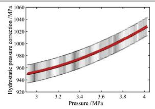
**Figure 4.** The hydrostatic pressure correction of the <sup>3</sup>He melting pressure thermometer during calibration at 1.2 K, together with standard uncertainty bars.
