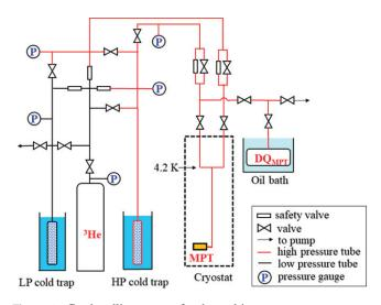
**Figure 2.** Gas handling system for the melting pressure thermometer.  $DQ_{MPT}$ : digital resonant quartz manometer; HP: high pressure; LP: low pressure.
