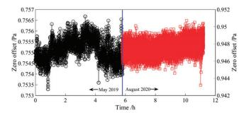
**Figure 9.** Zero offset of MKS Baratron 670B pressure gauge in May 2019 and August 2020.
