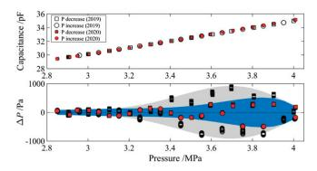
**Figure 7.** The graph in the upper part of the figure shows the capacitance measured as a function of the applied pressure at 1.2 K in 2019 and 2020. The lower part shows the corresponding fitting residuals of the eighth-order calibration polynomial. The blue and light grey shaded regions show the estimated uncertainty due to the hysteresis of the MPT capacitance gauge.
