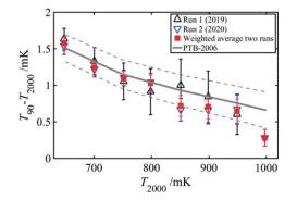
**Figure 13.** Values of  $T_{90}-T_{2000}$  from 0.65 K to 1 K from the present work and a comparison with the results obtained at PTB in 2006 [16]. The dashed lines correspond to the combined standard uncertainty of PTB2006.
