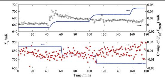
**Figure 10.** The effect of heating of the pressure tube on the value of the difference  $T_{90}-T_{2000}$  at 650 mK. Top: heating steps applied for increasing temperature during run 1 (2019). Bottom: steps applied for decreasing temperature in run 2 (2020). The temperature  $T_3$  (solid blue lines) corresponds to that of heater 3 shown in Figure 1. The difference in the sharpness of the steps between both figures is due to improved temperature regulation in the 2020 experiment.
