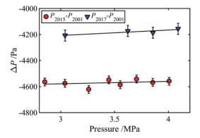
**Figure 5.** Offset of  $DQ_{MPT}$  with respect to its 2001 value, checked in 2015 (lower circles) and 2017 (upper triangles). The solid lines are least-squares fits to a linear function (slopes given in text).
