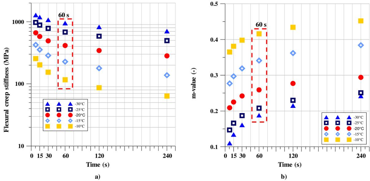
Figure 7. a) Flexural creep stiffness  $S(t)$  values for pure bitumen; b) Values of the slope of the stiffness versus time curve,  $m$ -value, on pure bitumen
