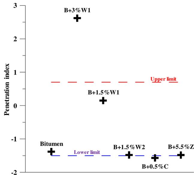
Figure 6. Penetration index for the six bitumen blends
