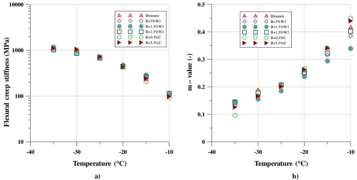
Figure 8. a) Flexural creep stiffness values on bitumen blends; b) Values of the slope of the stiffness versus time curve, *m-value*, on bitumen blends
