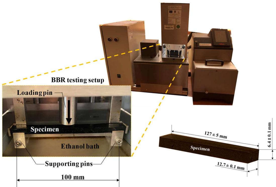
Figure 2. Bending Beam Rheometer test principle
