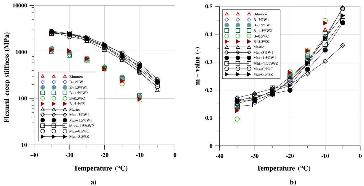
Figure 9. a) Flexural creep stiffness for bitumen vs bituminous mastic with or without additives; b) The value of the slope for bitumen vs bituminous mastic with or without additives
