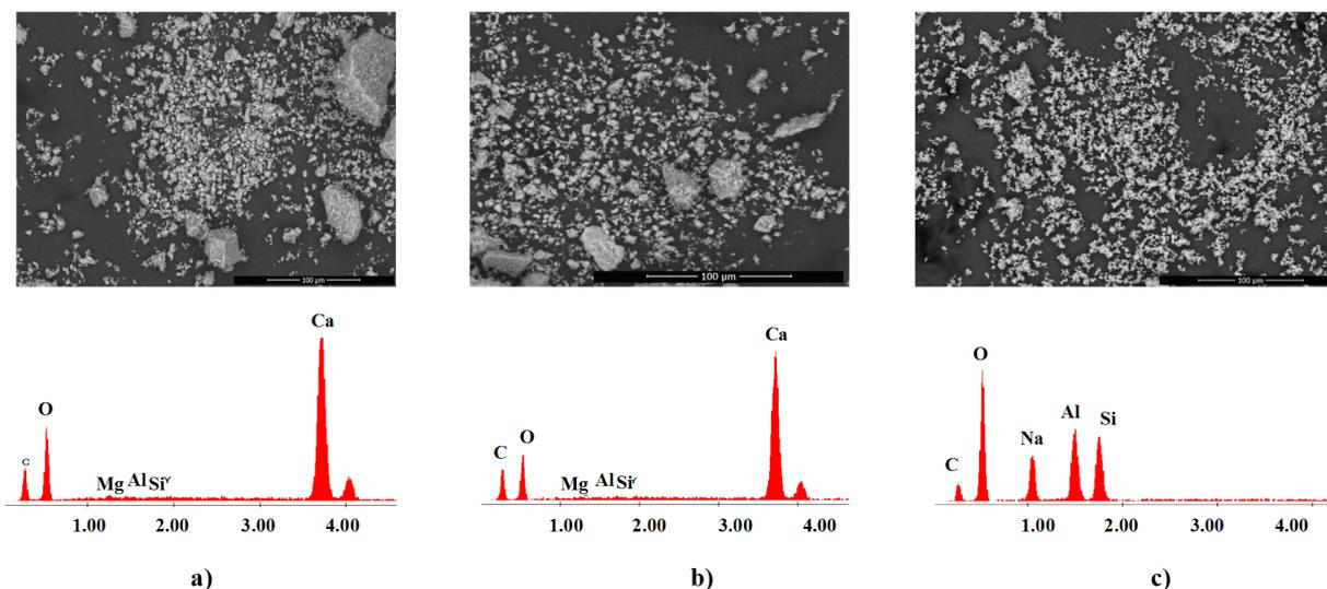
Figure 1. The morphology and elemental composition of: a) Filler; b) Filler blended with chemical additive; c) Synthetic zeolite
