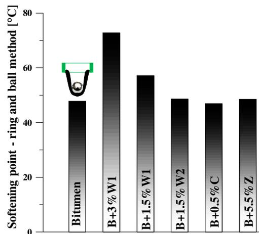
Figure 4. Softening point – ring and ball method
