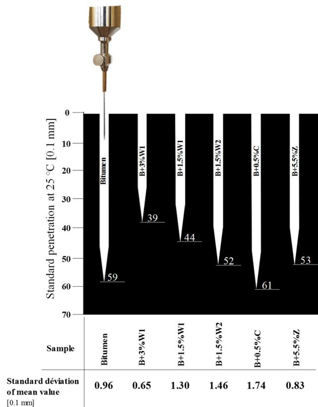
Figure 3. Results of penetration test
