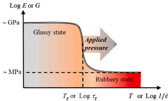
Fig. 1. Tensile or shear modulus as a function of applied temperature ( $T$ ) or strain rate ( $\dot{\epsilon}$ ), influence of applied pressure on glass transition or frontier between glassy state and rubbery state.  $T_g$  and  $\tau_g$  are the glass transition in terms of temperature and characteristic time respectively.
