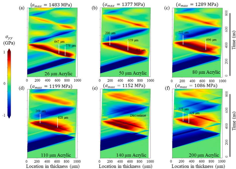
Fig. 10. Axial compression and tensile stress level  $\sigma_{yy}$  (blue and red colors respectively) during the wave propagation through the Pure Al sample (horizontal axis) and during the laser shock loading under  $1.8 \text{ GW/cm}^2$  for different acrylic thickness (26  $\mu\text{m}$ , 50  $\mu\text{m}$ , 80  $\mu\text{m}$ , 110  $\mu\text{m}$ , 140  $\mu\text{m}$  and 200  $\mu\text{m}$ ) in (a), (b), (c), (d), (e), and (f) accordingly.
