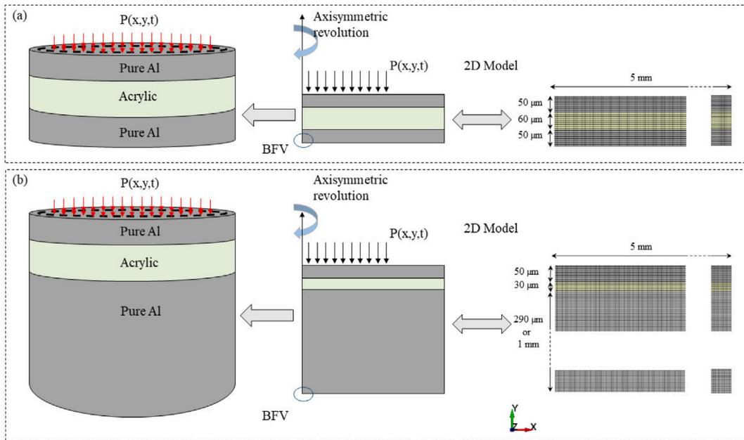
Fig. 4. 2D axisymmetric model for two configurations. (a) sample made of two aluminium tape, (b) made of aluminium tape attached on thicker Pure Al sample (290  $\mu\text{m}$  and 1 mm).
