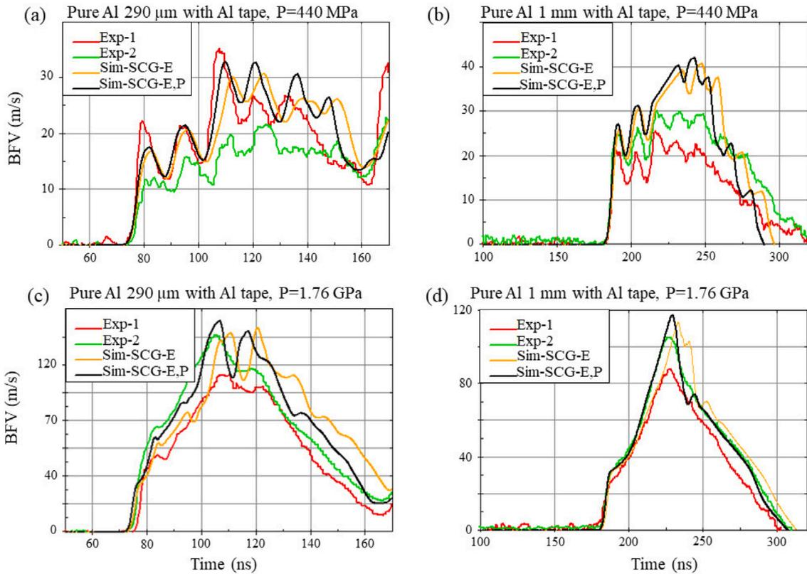
Fig. 6. Validation of the Simulated BFV for the taped Pure Al for two substrate thicknesses 290  $\mu\text{m}$  and 1 mm in (a, c) and (b, d) accordingly. Where the experimental results are the red and green curves (Exp-1 & Exp-2), the numerical response of purely elastic material model is the gold curve (Sim-SCG-E) and the black one is the elastic with pressure dependence numerical results (Sim-SCG-E,P).
