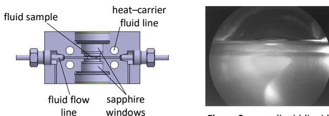
Figure 2. schematic description of the high-pressure microscopy cell
