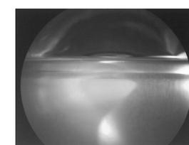
Figure 3. vapor-liquid-liquid equilibrium of the CO<sub>2</sub> + indane mixture in the UCEP vicinity ( $T = 313.1 \text{ K}$ ;  $P = 80.2 \text{ bar}$ )
