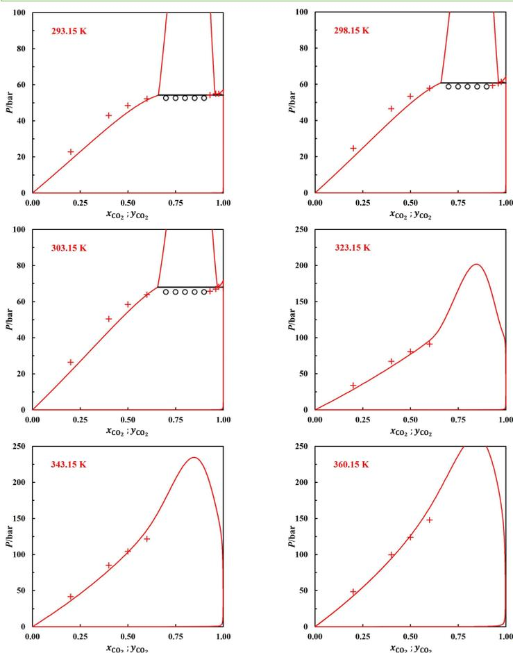
Figure 4. isothermal phase equilibria of the binary system CO<sub>2</sub> + indane
